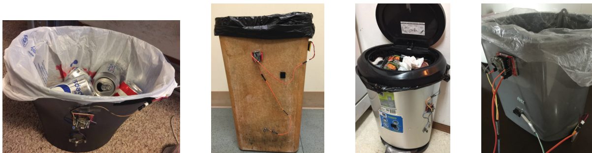
Fig. 5. Hardware prototype installation on the waste bins. We name them Bin1, Bin2, Bin3 and Bin7 from left to right.
